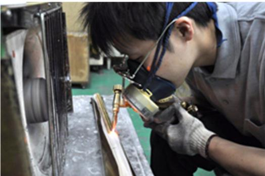
The connecting edges are lined up and seamlessly welded together with a 1000 C torch.
