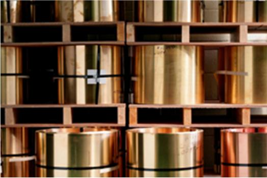
Rolls of metal sheet stock are sorted by brass, bronze, and silver alloy and utilized in different combinations depending on the saxophone model being made. Each roll is about 30 meters long.
