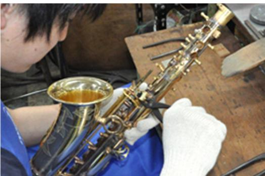
Preliminary key fitting is performed to enhance the precision fit of the key mechanism in the final assembly stage. The sax is also checked for silver-solder residues and flaws in the key mechanism.
