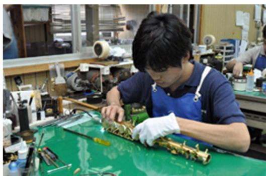
During assembly we apply a tape film to protect each instrument from scratches. Assembly proceeds with installation of the right-hand keys followed by the left-hand keys and then the side keys.
