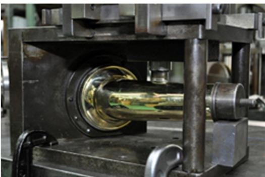
Tone hole locations are drilled into the shaped and polished body components after they are placed in a special die.
