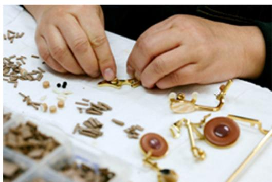
Pads and cork materials are installed on already-lacquered keys. We use three types of pad adhesive that vary by melting temperature. Also, to minimize the need for post-assembly adjustments, we use a composite resin cork that maintains its shape and firmness.
