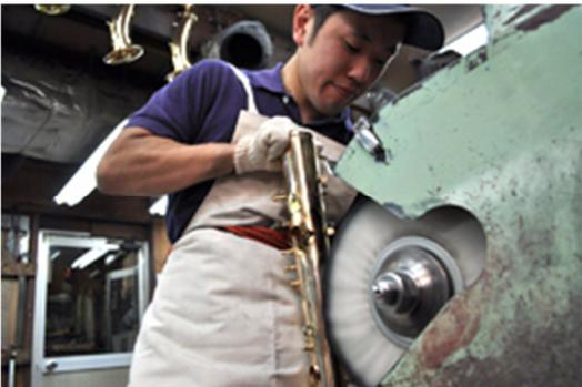
The body is polished in several steps with each pass utilizing a softer abrasive compound or buffing wheel.
