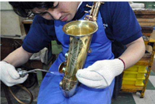
The bell and bow are soldered together, giving the sax its basic form.
