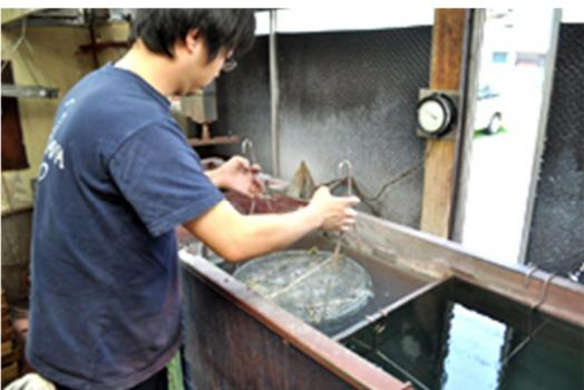
Prior to lacquering, everything is given an ultrasonic bath. This cleaning process completely removes all oils and buffing compound residues.
