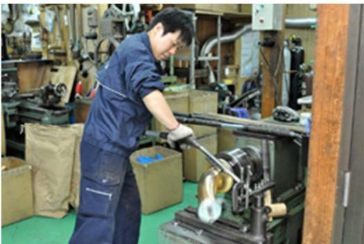
Sections of the bell that cannot be shaped by machine are spun on a lathe and shaped with a variety of handheld spatula tools.
