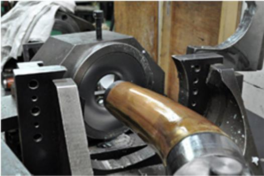
A metal mold is used to shape the body . An inserted tool forces the body through a slightly smaller-diameter hole in a metal plate. The hole in the plate is adjusted for changes in body taper.
