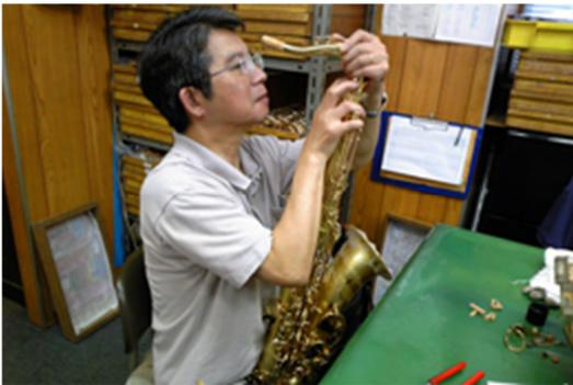
The instrument-making process concludes with a final, meticulous inspection of each fully assembled instrument. This inspection includes balancing the keys, tensioning the springs, and precision-fitting the neck.
