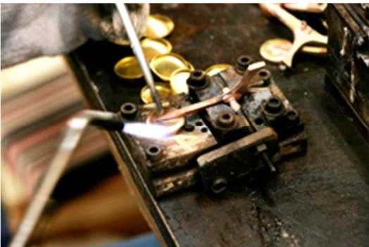
Over 120 different types of parts are created by silver-soldering key cups and other components to sax hinge rods and hinge tubing.
