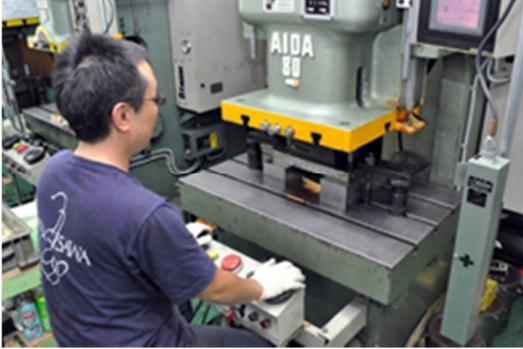
Sax key parts and certain body components are punched out on press machinery. Over 10 variations in thickness are used for such punched-out parts.
