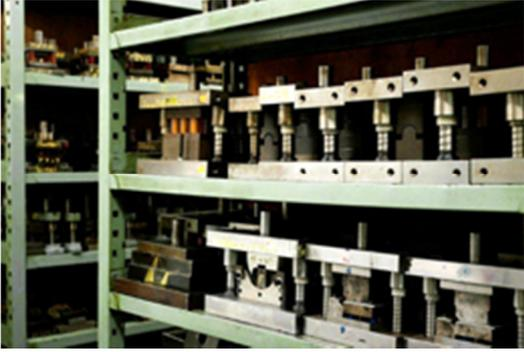
An assortment of press dies used to make various parts. Multiple dies are used in the production of each individual part. The factory uses over 2,000 dies in all.
