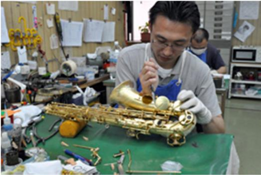
The assembly process is complete when the bell is attached to the instrument and the low-note bell keys controlled by the left-hand little finger are finally installed and regulated.
