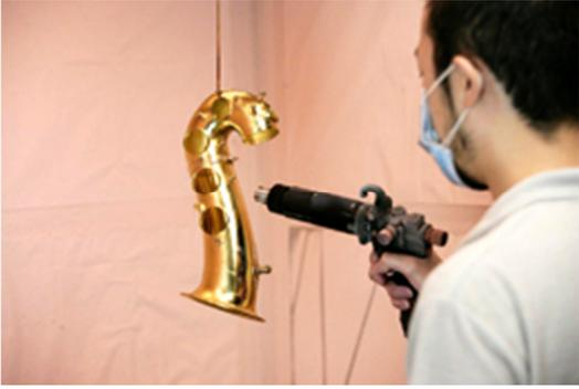
All parts are sprayed with a lacquer coat and then placed in an oven to heat-cure the lacquer.
