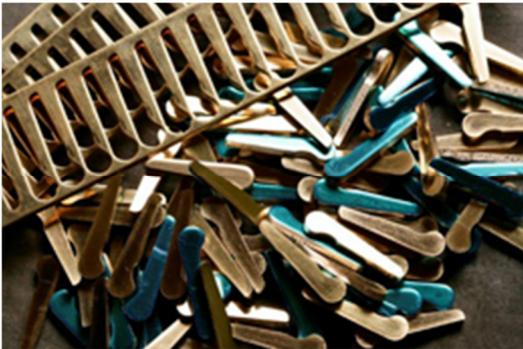
Parts initially punched out with press machinery also go through fabrication stages that involve drilling, bending, and shaping operations.
