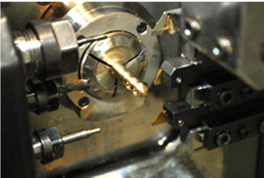
Sax posts of different sizes and shapes are cut to precision dimensions on CNC lathes.
