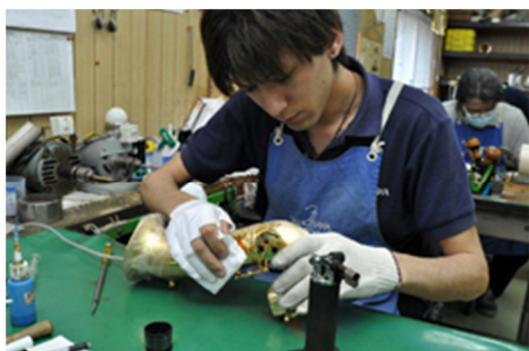
Using a leak light, each pad seat is checked for air leaks and adjusted as necessary.
