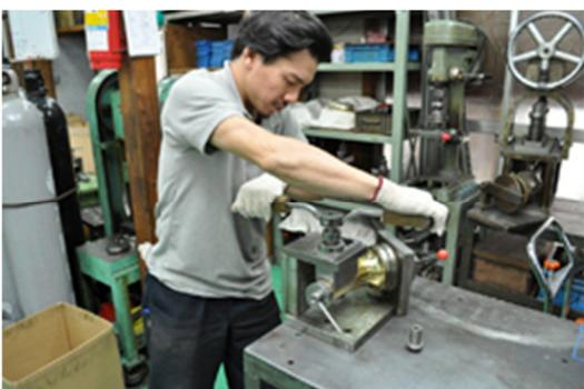
When the handle is turned, a round piece is pulled through to form and draw out the tone hole from the wall of the body tubing. Special care is the rule when fabricating tone holes because they have the most significant influence on the saxophone's scale.
