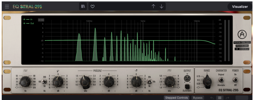
EQ SITRAL-295 Mono configuration with Visualizer opened. Notice the Auto Gain switch under the Output control knob.
