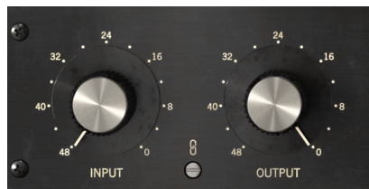
Comp FET-76 Input and Output controls at the default position. We may see the Link switch in the bottom, between the two knobs
