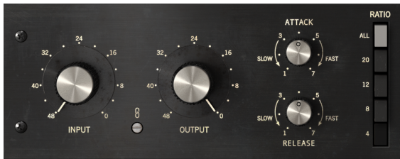
The Main FET-76 Compressor Controls
