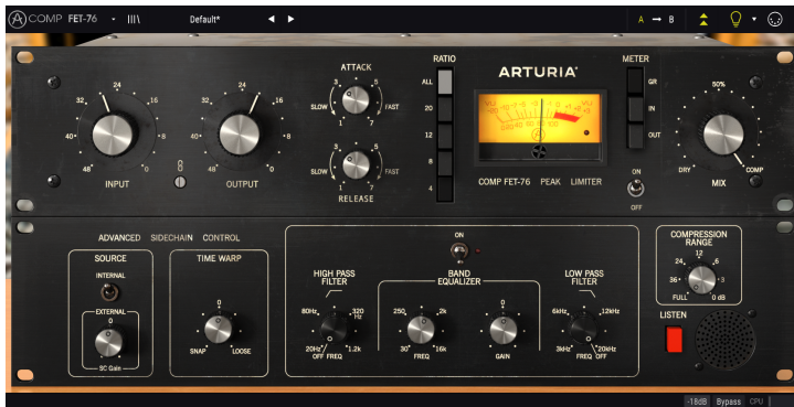
Comp FET-76 inserted in a mono track. Notice the absence of the Detection Mode selection control knob
