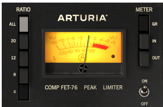
Comp FET-76 VU Meter, set to Gain Reduction. Notice the letter L in the lower left corner and the clipping LED indicator in the lower right corner.
