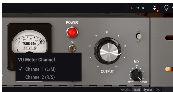
VU Meter channel selector. In the Lower Toolbar we can see the calibration set to -18 dB
