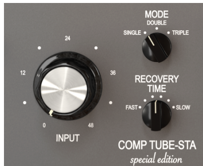
The Main Tube-STA Compressor Controls
