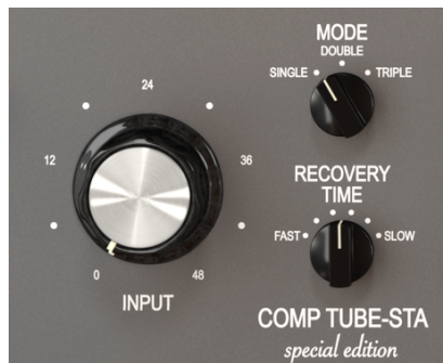
Main Compressor controls in STA Tube Compressor
