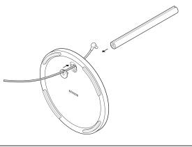
Fasten the base (with the washer) tothe stand pole using 1 long screw(included) and a Phillips-headscrewdriver. Make sure the cord canstill slide freely.
