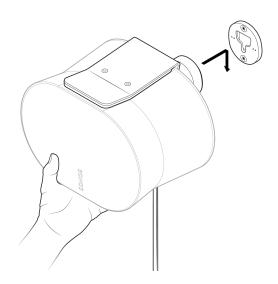
To adjust for optimal sound, unlock the speaker by rotating the collar on the mount 90° counterclockwise. Reposition the speaker, then rotate the collar 90° clockwise to lock.
