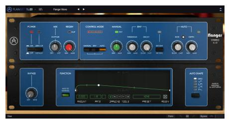
When instantiated as mono-to-stereo, you have the Stereo Offset control and the Reverse Sweep O/P 2 switch, but the Mono/Stereo button is not present, since the source signal is mono. Bear in mind that, when used with mono sources in the mono-to-stereo configuration, the source signal remains mono, but the processed signal will have some stereo definition and depth, hence the presence of the other two controls.
