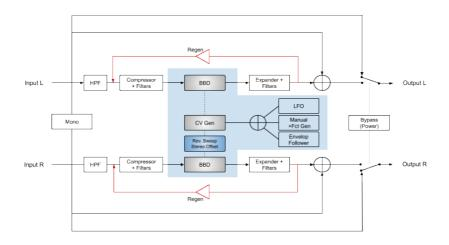
When the plug-in is bypassed, the input signal is routed directly to the output. This is the signal heard when you press the Power button or the Bypass button in the Lower Toolbar.
