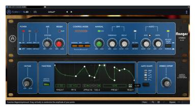
Flanger BL-20 after playing with the Regen feature a few times. We also have pressed the three Control Mode buttons, the External Envelope button and the Reverse Sweep button to show some extra options, although so far, we have only used a single mode at a time. The selected waveform in the Auto Shape is the square, which we found great for getting stereo pingpong effects.
