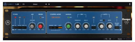
Notice that each time you click a control (knob or button), or simply hover the mouse over it, the Lower Toolbar displays the parameter name at the lower left. Also, a small pop-up box appears to the right of the control displaying the current parameter value. This changes every time you move that control, updating the parameter value in real time.
