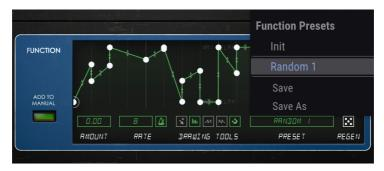
The Preset menu of the Function generator, showing the saved function shapes.
