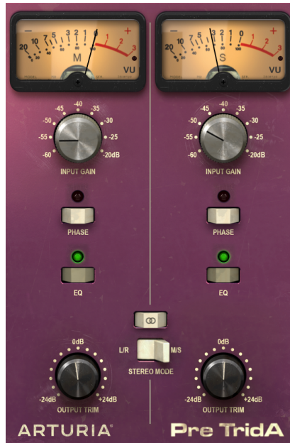
The TridA preamp section configured to work in M/S mode. Notice the Stereo Link switch turned Off and the Stereo Mode switch in the M/S position.
