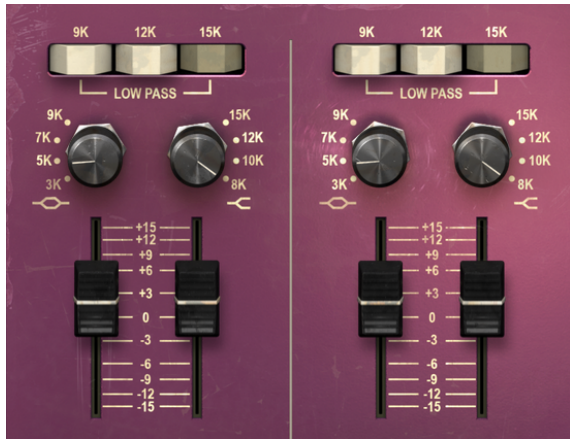
TridA Double Channel EQ upper bands (High Shelf and High Midrange Bell), and the three Low Pass Filter switches on Top
