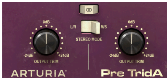
TridA Double Channel Output Trim knobs and the switches to control the Double Channel behavior (Stereo Link and Stereo Mode)
