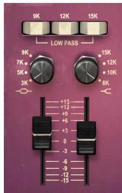
TridA Single Channel EQ upper bands (High Shelf and High Midrange Bell), and the three Low Pass Filter switches on Top
