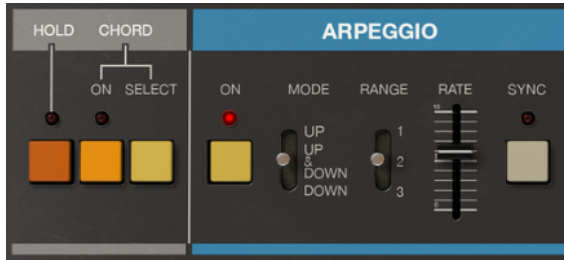
Jun-6 V Hold button, the new Chord Selector and Chord button (added by Arturia), and the Arpeggiator controls, including the new Sync button also added by Arturia.
