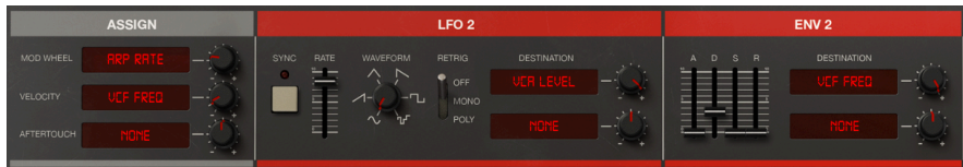
Jun-6 V advanced modulation sections, including the mini modulation matrices, LFO 2 and Envelope Generator 2.
