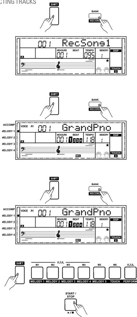
The track indicators on the display have three states: blinking, light on or light off.
