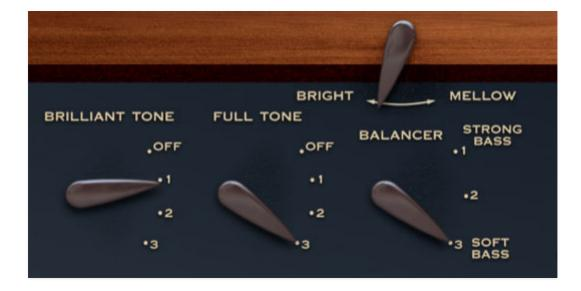
**Brilliant Tone**- Sets the level of tone generator signal with a one-pole (6dB per-octave slope) highpass filter with a fixed frequency of 2000 Hz applied.
