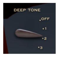
**Deep Tone**- Sets the level of tone generator signal with a one-pole (6dB peroctave slope) lowpass filter with a fixed frequency of 160 Hz applied.
