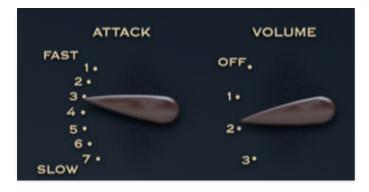
**Attack**- Unlike a typical synthesizer ADSR-style attack control that only affects the onset of the amplitude curve, Novachord's *Attack* lever shapes attack, decay, and sustain amplitude characteristics (release is "instant-off" like an organ at all settings).
