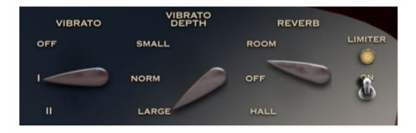
**Vibrato**- Enables the Novachord's unique vibrato circuit. *Vibrato I* uses square-wave modulation, as used in the earliest Novachord models; *Vibrato II* makes use of a more rounded-off mod wave, as used in later Novachords.
