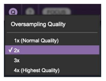
**Q Oversampling Quality -** The Q button sets Novachord's internal oversampling rate; the higher the setting, the better audio fidelity will be, with the caveat that more computer processing power will be required.
