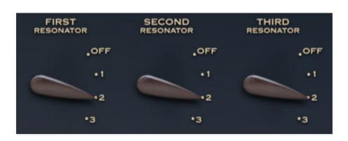
The three resonators are bandpass filters, operating consecutively in low, mid, high frequency ranges.
