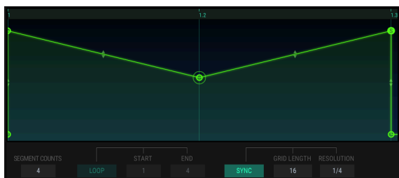
An added point will be quantized to the nearest quarter note when the Resolution is 1/4 .
