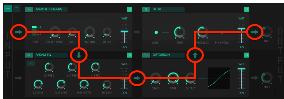
Signal flow of the FX chain in series mode
