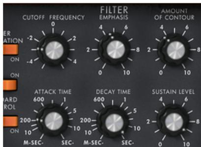
*Lower the cut-off frequency of the low pass filter*
