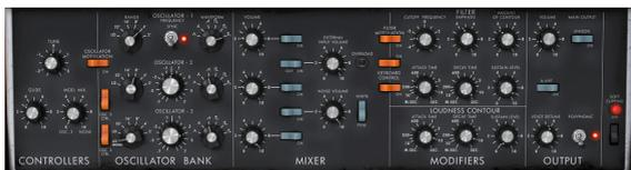
So as to hear the sound, click on the first of the 5 blue “Mixer” switches. This activates the signal coming from the first oscillator.
