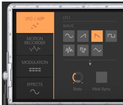
On the original synthesizer (equivalent to the “Classic” mode), oscillator3 can be set to the low frequency (“Lo” position in the range) to be used in LFO mode. This removed the possibility of using 3 simultaneous oscillators as well as a slow modulation on the filter cut-off frequency for example.
