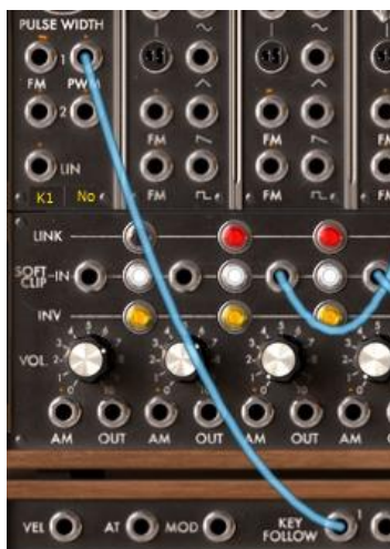
Connection of the PWM to the key follow input 1 (key follow1)
