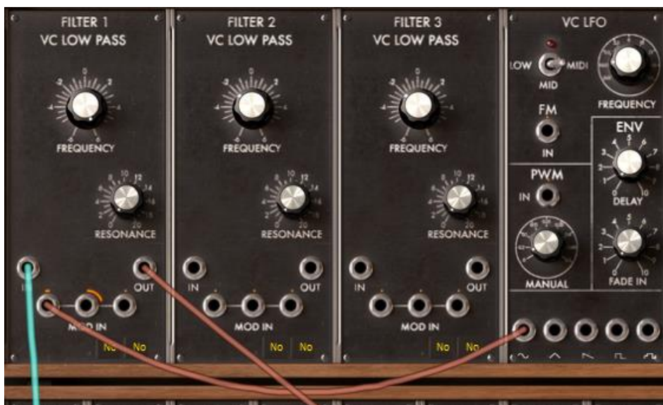
Connection of LFO to filter1
