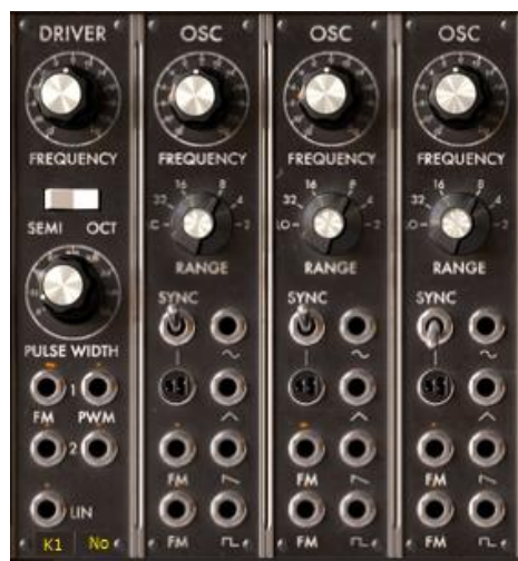
An oscillator bank: 1 “driver” and 3 “slave oscillators”
