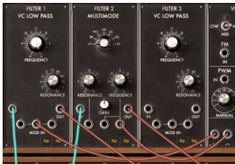
LFO1 to the filters link
