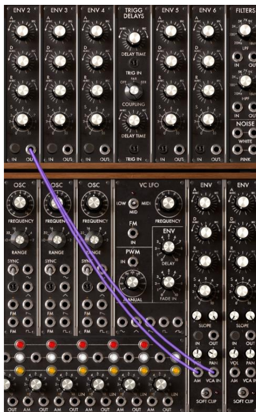
Connection of an auxiliary envelope for the output VCA
