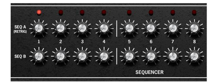
**Seq A (Retrig)** / **Seq B CV knobs 1-8**- These set the CV amount for each stage sequencer stage. The CV range depends upon the settings of the *Range* switches. *Seq A* and *Seq B* CV settings are independent, but the stage (step) number is always locked together for both. The lamp above each stage indicates the current stage.
