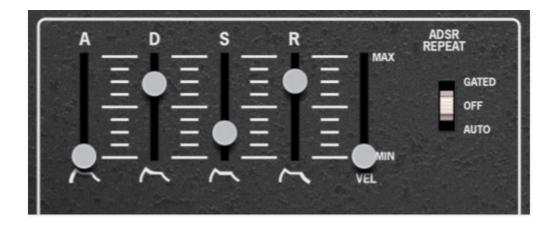
A (Attack)- Defines the length of time for voltage to rise from 0V to 5V when a key is played.
