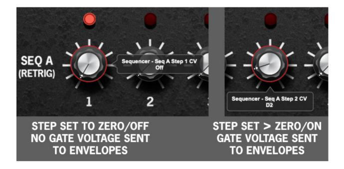
**Disabling Gate Voltage for Seq Stages** - Setting any of Seq A's knobs to minimum disables the gate voltage for that stage. This allows you to disable stages, enabling far more interesting musical phrases and is why Seq A is labeled (Retrig) beneath. Note that Seq B CV knobs have no effect on gates/note triggering.
