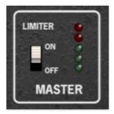
**Limiter**- The *Limiter* switch applies a transparent limiting effect to help prevent overloading. This is particularly useful with higher *Number of Voices* settings.
