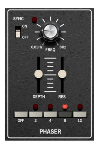
**Sync**- The *Sync* slide switch locks the rate of the Phaser's modulation LFO to the tempo in the top toolbar when using The Cat standalone version, or to the current project tempo when the plug-in version is used in a DAW. When
