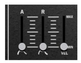
**A (Attack)**- Defines the length of time for voltage to rise from 0V to 5V when the gate voltage is applied.
