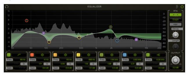
The Equalizer module consists of a 5-band EQ with 2 additional filter bands, an **Output Trim** control, and an optional **RTA display**. Each band has adjustable Frequency, Gain, Shape, and Q parameters as well as the option to toggle it in or out. You can control the bands directly on the **EQ Graph** or with their corresponding controls below the graph.
