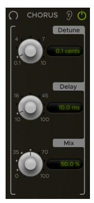
The Chorus is an effect that can be used to boost overall presence and add some extra flare to a bass signal. It has Detune and Delay controls for dialing in the effect and a Mix control for blending it with the dry signal.
