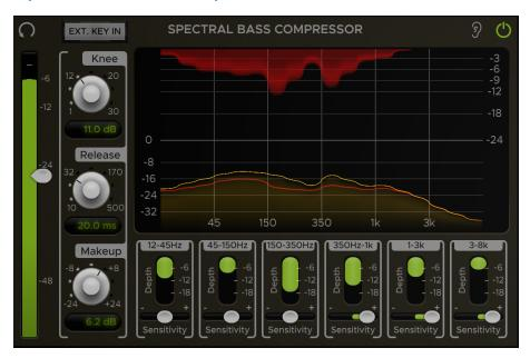
The Spectral Bass Compressor is a multiband compressor designed especially for bass. It allows for applying compression selectively across 6 frequency bands focused in the lower end of the spectrum where bass notes mainly reside.
