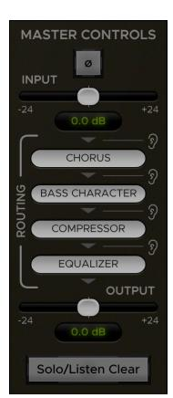
The Master Control section at the bottom-right corner of the plugin window contains controls for switching input polarity, adjusting input & output trim, and setting the order of routing between elements.
