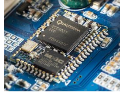
Bluetooth Wireless HD Qualcomm aptX HD supports 24-bit music quality over Bluetooth
